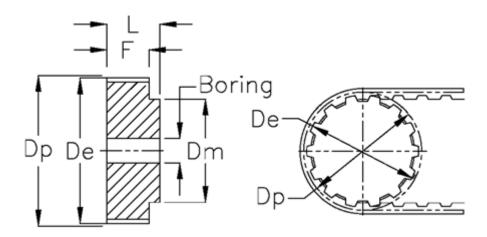
Type = T10Belt width = - 25 mm Weight = 2.339= 189.1 De Dm = 110 = 191.15 Dp F = 30 L = 40 Pre-drilled = 16 Tooth number = 60
